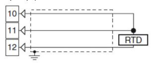
**Calibration:** According to EN 60751/A2. The resistance of the 3 wires **must** be the same.
