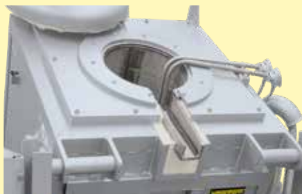
Tilting furnace for heavy metals with bath control
