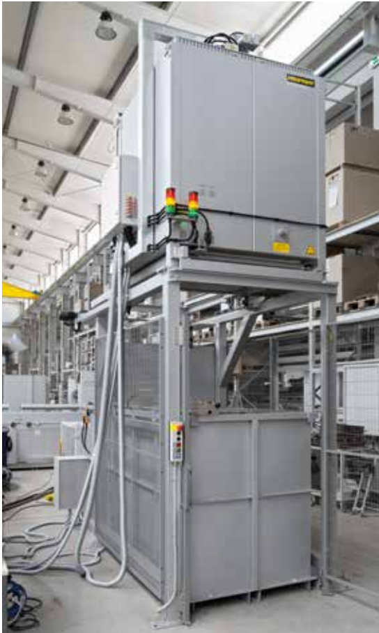
Drop-bottom furnace with fixed quenching bath
