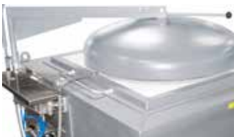
Melt bath control with a thermocouple in the melt
