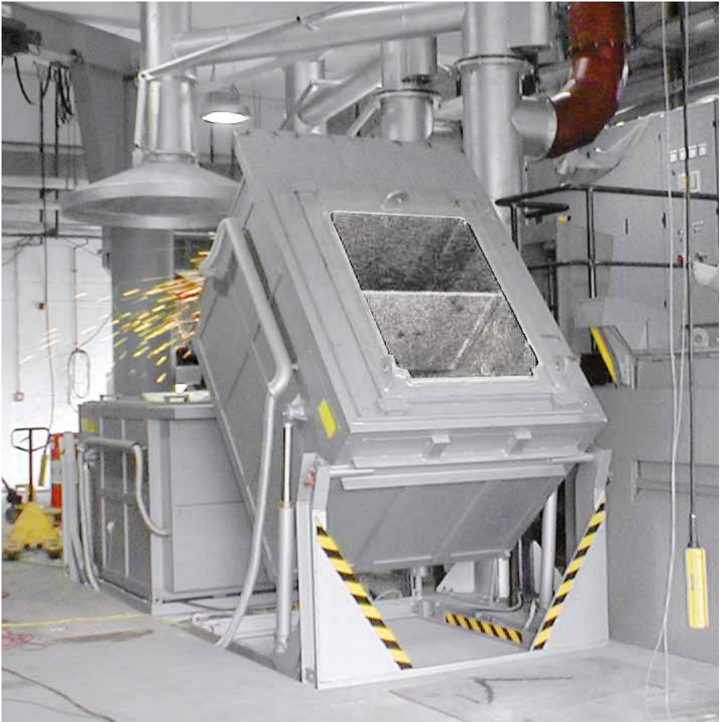
Tilting furnace K 1500/75 S for magnesium with 1500 liters crucible volume
