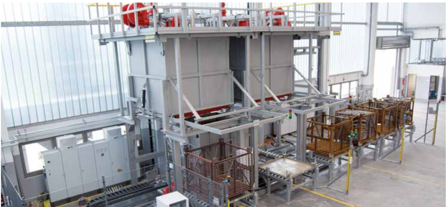
Fully automatic drop-bottom furnace plant, consisting of two drop-bottom furnaces, movable water bath and several loading and unloading positions
