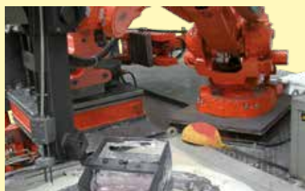
Bale-out of bale-out furnace with robot
