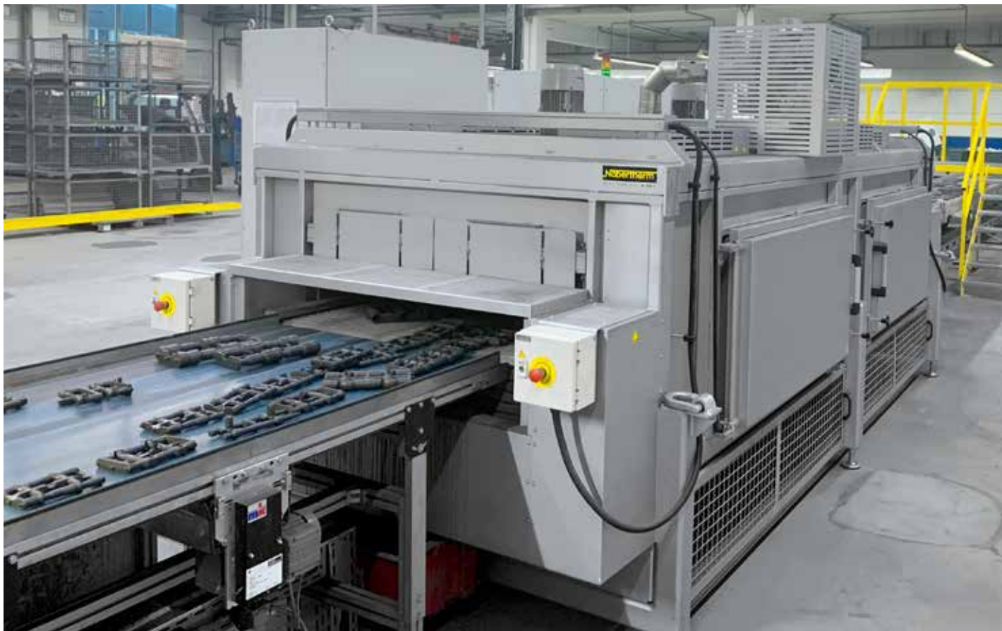
Continuous belt furnace D 1000/4000/140/35 AS for black wash drying on sand cores
