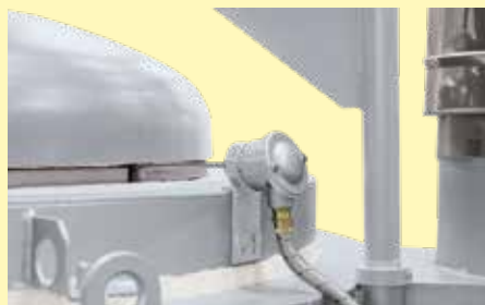
Thermocouple for melt bath control
