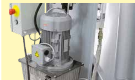
Hydraulic system with flame resistant hydraulic fluid
