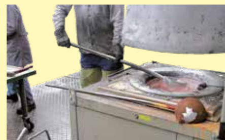
Manual ladling from a bale-out furnace T 80/10
