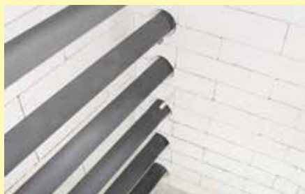
Heated on both sides by high performance SiC rods
