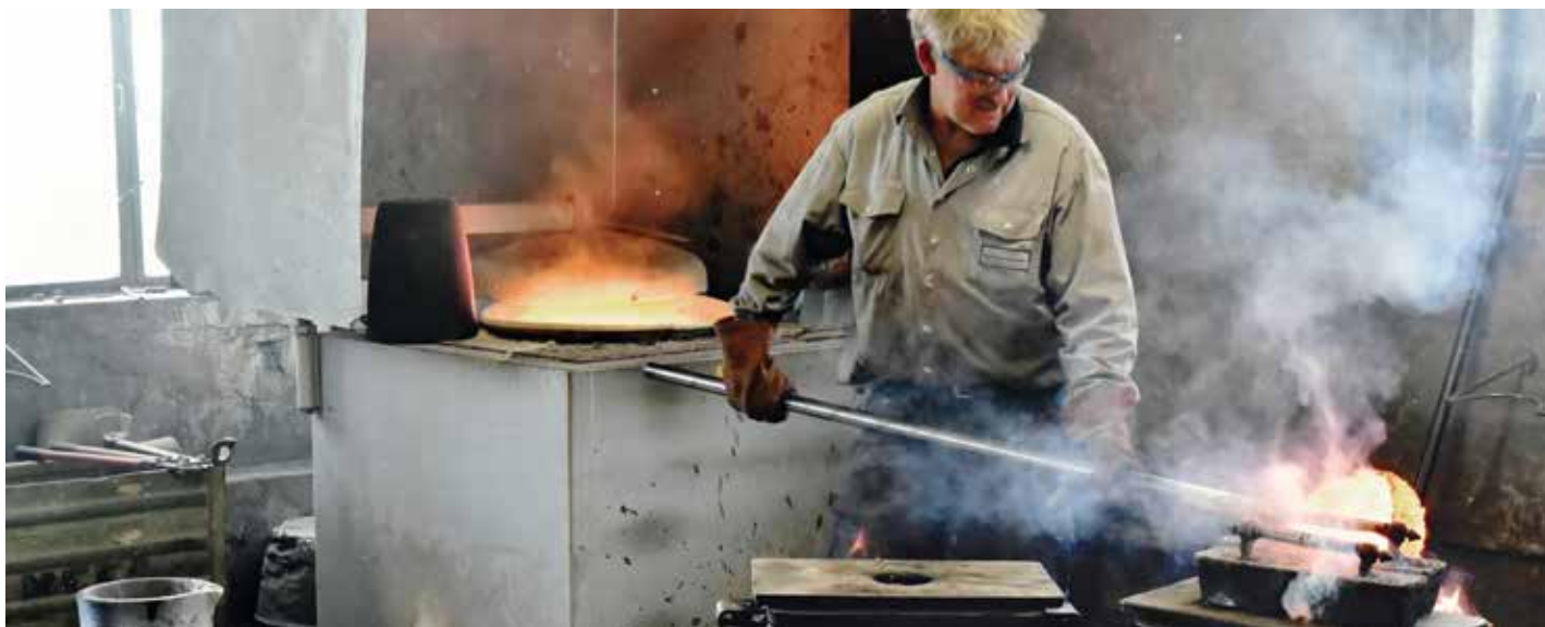
Bale-out furnace T 80/13 for gunmetal in a sand foundry shop
