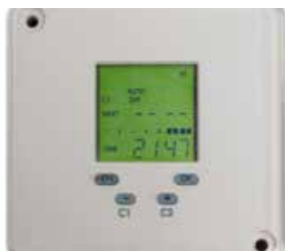
Weekly timer to switch between melting temperature and lower temperature
