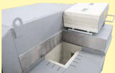
Inlet opening for filling with liquid aluminum
