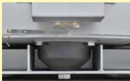
Forklift entry with dampers
