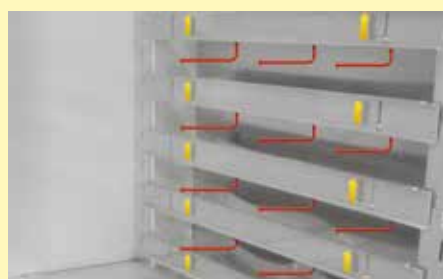
Adjustable plate shutters to adapt the air guide to the charge
