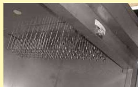
Enclosed heater coils on electrically heated models
