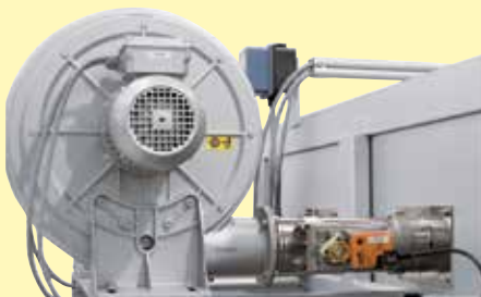
Cooling fan for accelerated cooling
