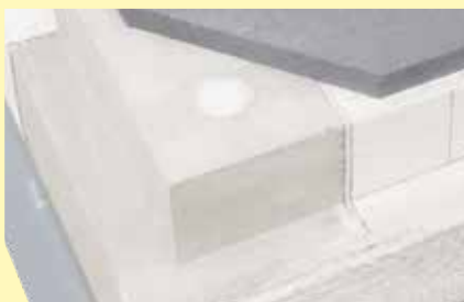
Thermocouple inlets (Ø 40 mm) in the front corners of the bogie
