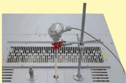
Thermocouple port in the ceiling with tripod
