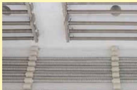
Fiber insulation to reduce heating and cooling times
