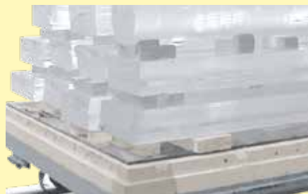
Bogie hearth furnace for tempering quartz rods
