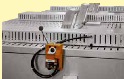
Motorized exhaust air flaps as additional equipment
