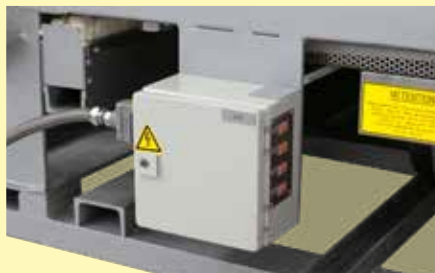
Charge thermocouples with plug-in connection
