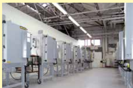
Chamber furnaces N 200/14 for sintering semiconductors
