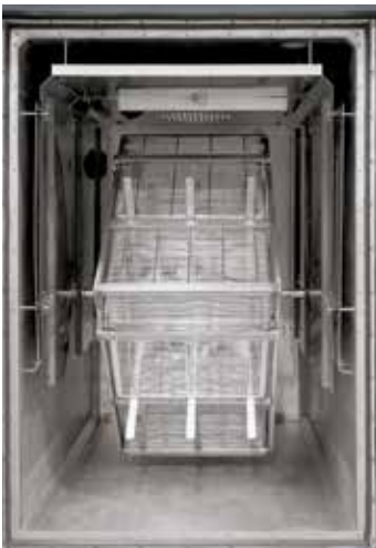
Motor-driven rotary rack with baskets for moving the charge during heat treatment
